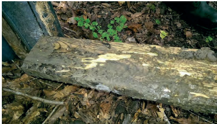
Figure 3. Evidence of Formosan termite feeding on the feeder stake.
